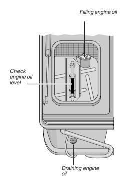
There are three plugs for draining. One on the bottom edge of the dry sump, one by the oil pocket on the inspection hatch and one on the bottom of the oil reservoir. The engine oil reservoir is located in the rear right corner of the bus.
