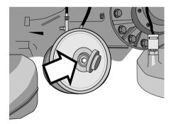
Mechanical release of handbrake
