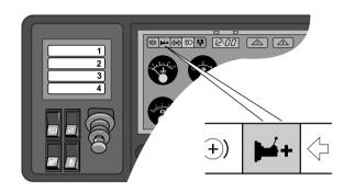
The indicator lamp goes on when high range is engaged
