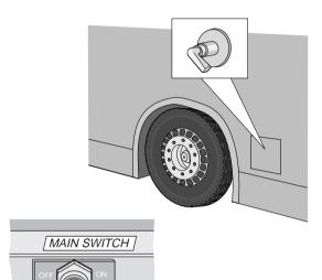
The battery master switch must be in the on position for the electrical system to work. A common coach-builder solution is to place the knob for the battery master switch by either the passenger door or by the drivers seat.
