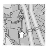
The plug is located in the engine block close to the flywheel cover.
