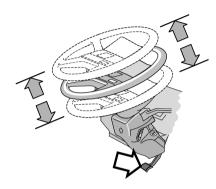
The height of the steering wheel is adjusted to the desired position by pushing down the pedal while at the same pulling up the steering wheel or pushing it down.
