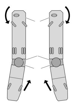
Direction of trailer coach wheels when steering left alternatively right (steered trailer coach)
