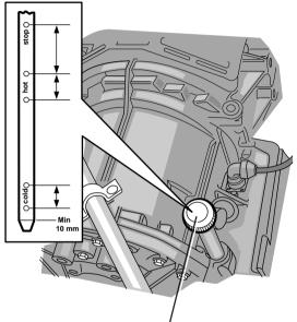
When checking level and topping up, make sure the vent holes in the cap are
