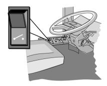
Other types of battery master switches may also be present, i.e. a toggle switch placed on the side panel by the driver's seat or a switch behind the cover to the front headlight on the door side of the bus. These switches work in the same way as the control knob, i.e. they are used to switch the battery master switch on and off.
