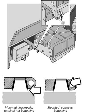
Battery lead terminal fitted to battery
