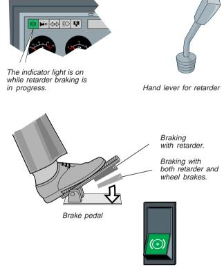
Switch to interrupt retarder activation via brake pedal
