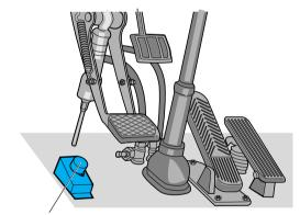
Switch for exhaust brake
