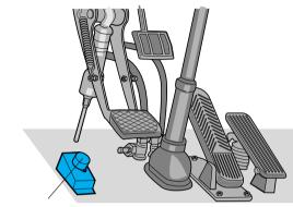
Switch for exhaust brake
