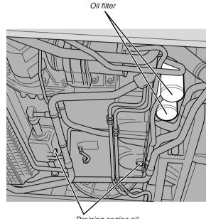
Training engine oil (+ a plug in the bottom of the oil reservoir, see text)
