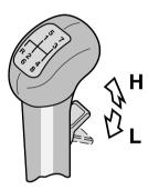
Low range should be engaged when reversing so that full control of the bus is retained.
